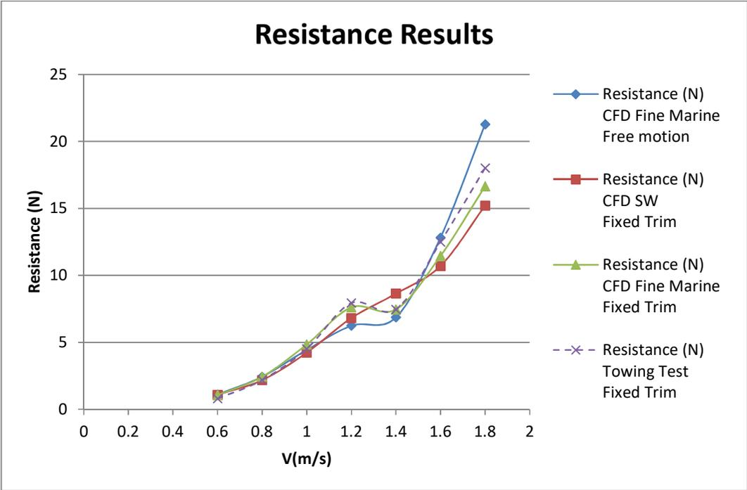
Figure 6 comparison of CFD and Towing test of ship resistance without appendages.
