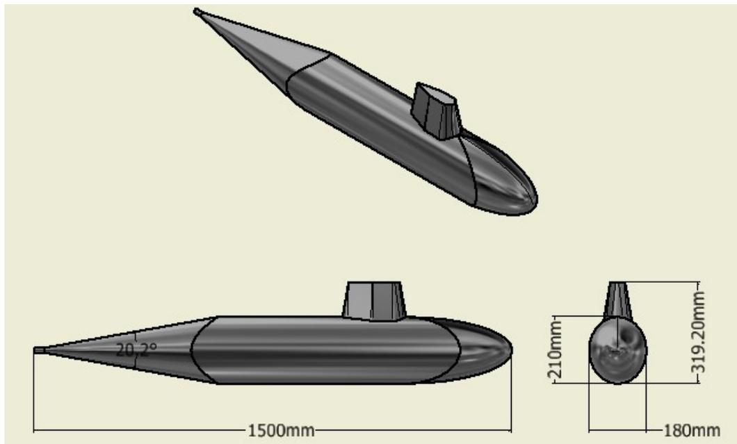
Figure 1 Model of underwater vehicle
