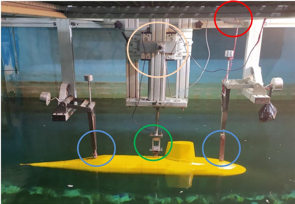
Figure 3 Towing mechanism arrangements
