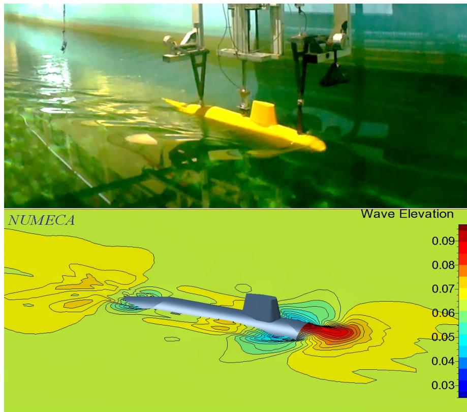
Figure 5(a) Towing tank test and CFD simulation with 0.8m/s
