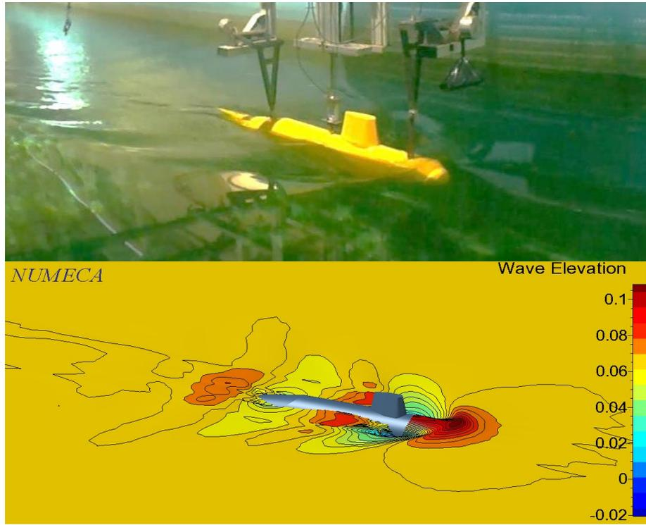
Figure 5(b) Towing tank test and CFD simulation with 1m/s
