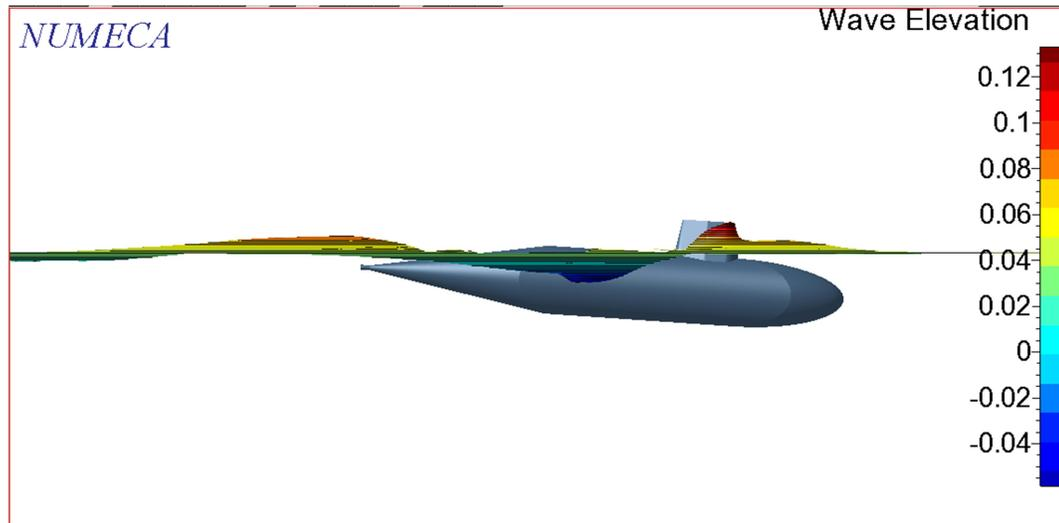
Figure 7 Hydrodynamic effect of the model (down force)
