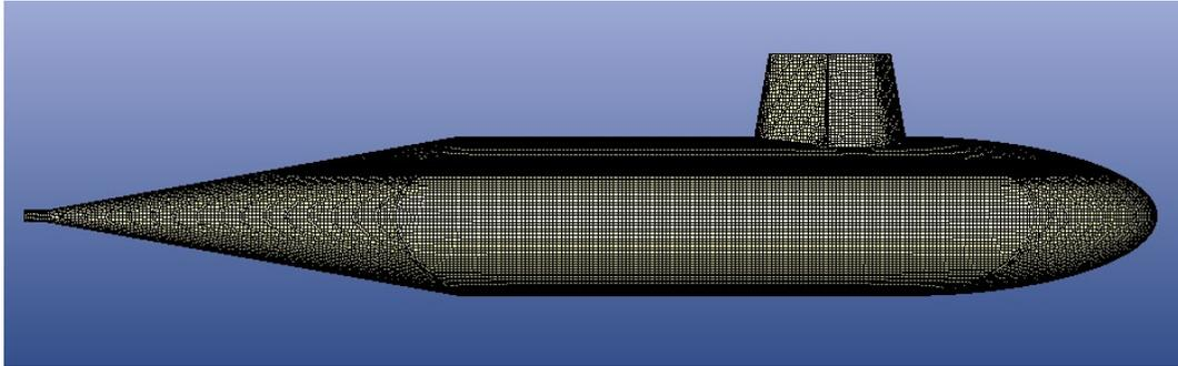
Figure 4b Generated mesh of model
